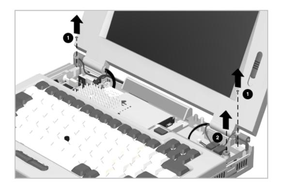
Figure 5-38. Removing the Keyboard Screws and Microphone
